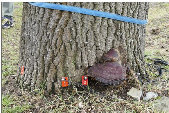
**Fig. 4.** Butt-end of trunk in tree no. 2 during a CT scan with a visible fruiting body, photo: M. Mincel
