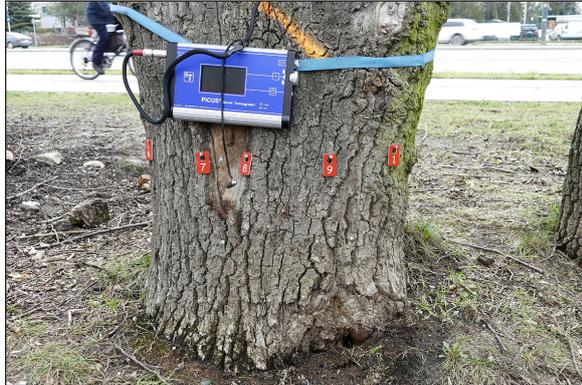
**Fig. 3.** Tomograph examination of tree no. 1, the butt-end on the right side has a visible trace of a fruiting body, photo: M. Mincel
