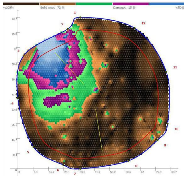
**Fig. 7.** Tomogram - tree no. 2, examination at a height of 10 cm
