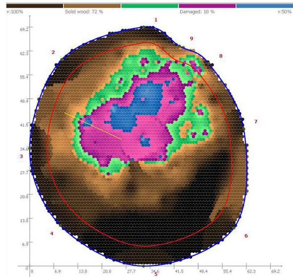
**Fig. 5.** Tomogram - tree no. 1, examination at a height of 4 cm
