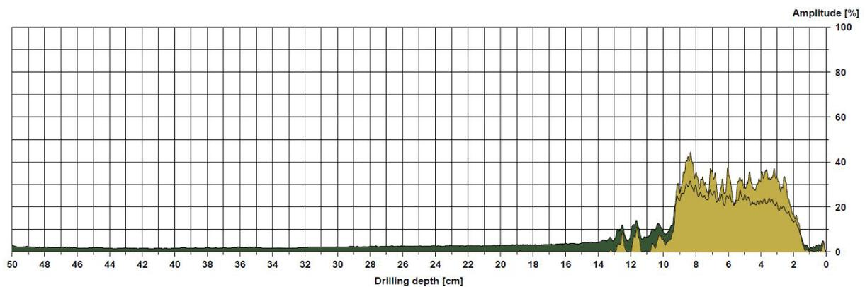
**Fig. 8.** Dendrogram - tree no. 2, examination at a height of 10 cm
